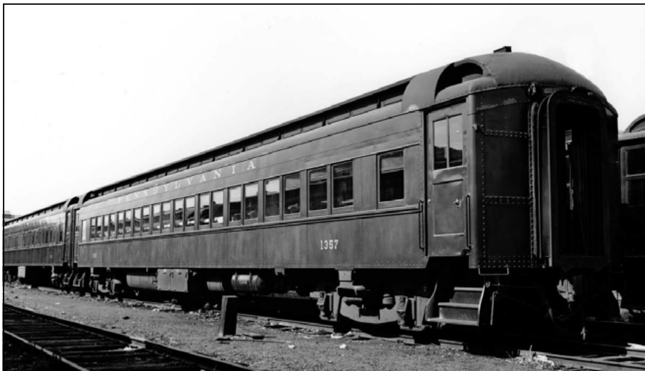
Pennsylvania Railroad heavyweight P70 coach car. Beginning early in the 20th century, the Pennsylvania Railroad authorized initial construction of the all-steel, 80' long P70-class heavyweight coach car. By the beginning of the Second World War, over one thousand P70s served on the PRR's vast fleet, although many had been rebuilt and modernized to meet customer demand. This car shown, #1357, had been built in 1914 for the Pennsy by the Standard Steel Car Co., photographed at Sunnyside Yard, Queens, in 1936, and remained with its spartan, old-style seating arrangement. In 1943, when the War Department required railroad companies to contribute specifically modified coaches for PW transportation, the PRR selected the older, non-modernized P70s, such as #1357, which by that time had been almost completely relegated to branch line service. Robert Liberstand Collection.
