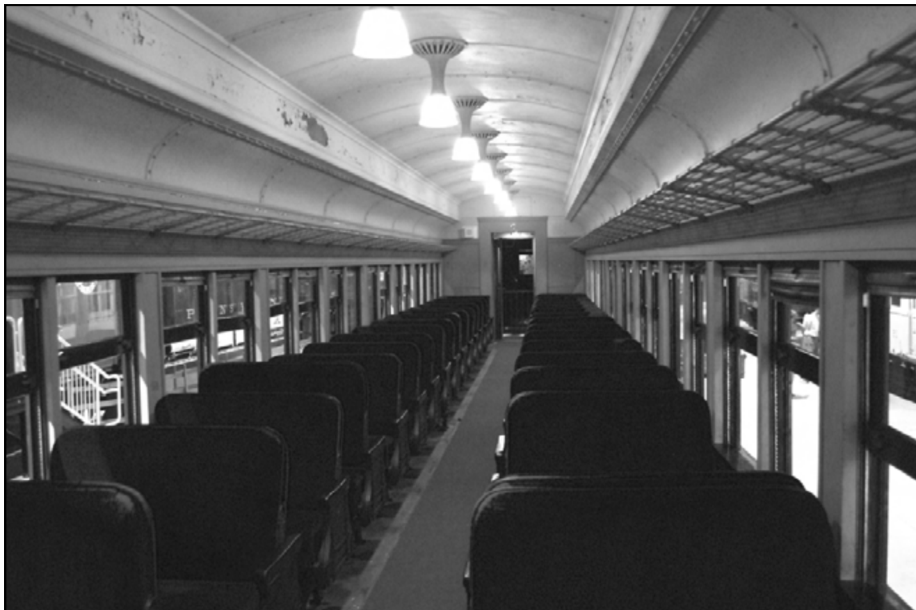
Interior of old-style, heavyweight P70 passenger coach. An example of a non-modernized Pennsylvania Railroad P70 heavyweight coach is #1006, today residing at the Railroad Museum of Pennsylvania in Strasburg. Originally built in 1928 by the Standard Steel Car Co. as PRR #3433, it still retains its old-style walkover seating arrangement with a maximum capacity of 88 passengers. Yet, “spartan arrangements” are in the eye of the beholder, and many a German PW marveled at this example of American luxury. Image provided by the author.
