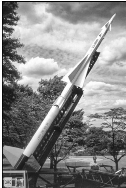
The Nike-Ajax missile, shown mounted for display upon its mobile launcher at a Phoenixville Memorial Day celebration in 1958, was only twelve inches in diameter and twenty-one feet long (thirty-four feet long with its booster attached). But upon launch the missile would reach a speed of almost 1,700 mph in less than four seconds before its booster fell back to earth. Courtesy of Tredyffrin Easttown Historical Society.
